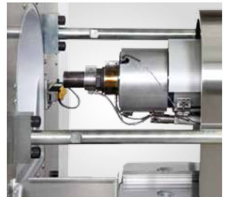
Optimized process control thanks to an actively controlled nozzle needle valve.
