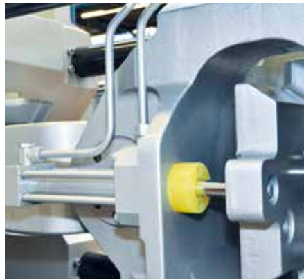
Hydraulic ejector activated with two parallel cylinders.
