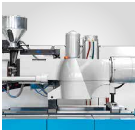
Dynamic, high-precision all-electric injection unit.
