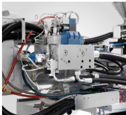
Dual-valve technology; maximum performance for injection movement.
