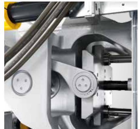
Electric ejector with precise and dynamically level activation.
