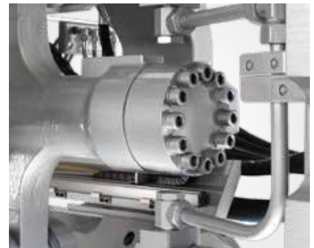
Reduced footprint thanks to inward-facing closing cylinder
