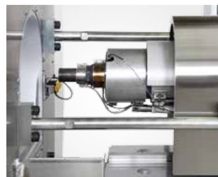
Optimized process control thanks to an actively controlled nozzle needle valve
