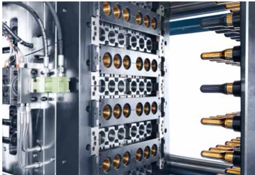
PET-LINE with mold for PRElactia® preforms
